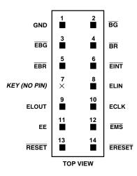
Figure 7. Target Board Connector for EZ-ICE
